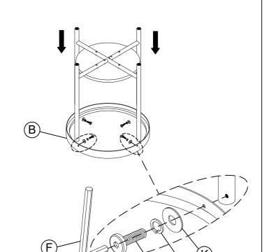
Step 3: Using the Allen key to tighten all bolts.
